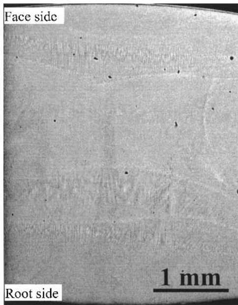
Fig. 5 SEM micrograph of the weld showing the face and the subsequent root-pass
